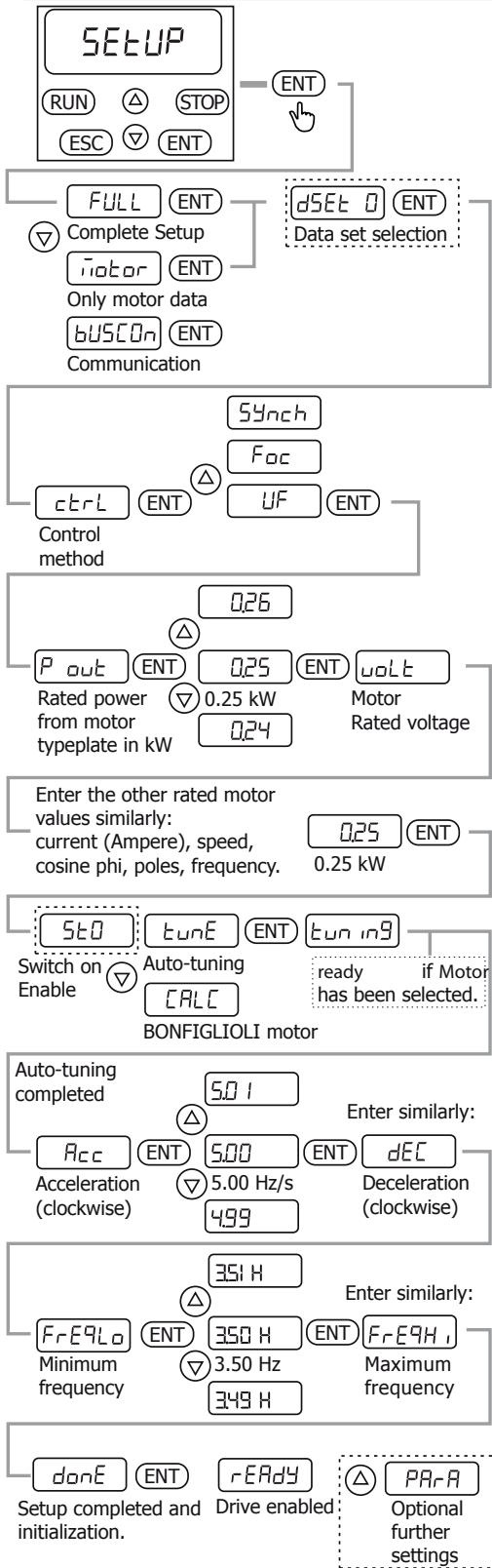
Setup can be selected via menu item "Setup". At first switch-on Setup is displayed automatically.
