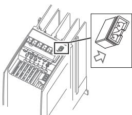
For connection on IT mains configuration remove the IT-jumper.
