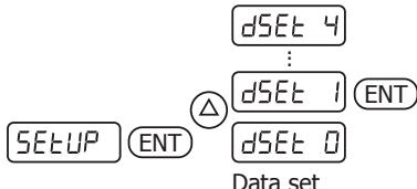
When setup is carried out the entered and measured motor data is stored in the selected data set.
